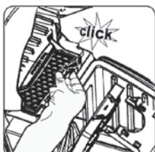
Put the HEPA in the machine and press to fix it
